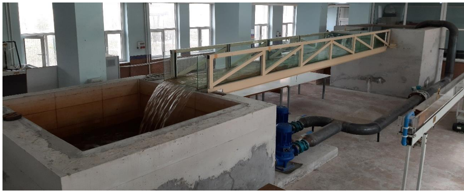
Fig. 3. Open channel system used in experiments.
